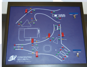
5. Complex Interior Desk-Mounted Master Control Panel
